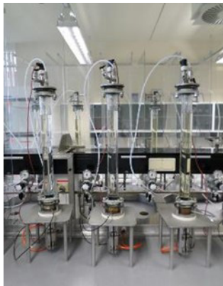
Test setup: ASTM D4340 Adapted to fuel cell operating conditions
